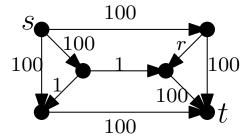
**Solution.** Consider the graph below with the given capacities.<sup>1</sup> The goal is to find a sequence of augmenting paths such that the algorithm converges to a value which is much smaller than the value of maximum flow.
